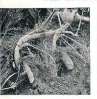
When clean plowing is a problem, the Weed Hook Assembly for Ferguson System Plows provides the necessary "hold-down" of trash and vegetation for complete coverage. The hooks attach to the plow beam by simple brackets. In operation, the moldboard turns the furrow slice toward the front hook and over the rear hook to guide and hold trash into the furrow bottom.
