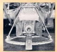
power take-off operated machinery by merely dropping a bolt through the drawbar and guide. Exclusive Ferguson Notched Guide Bar holds drawbar rigid during backing.
