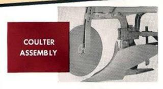
The Rolling Coulter and Shank Assembly are available for use with the Ferguson Middlebuster. Coulter splits ridges and cuts through stalks and surface trash that normally clog or drag on moldboards. Adjustable for a deep-working cut and sufficient penetration for the "busting-out" of flatlands. Easily attached and detached when converting Middlebuster to cotton and corn planter.
